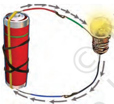
Fig.9.6 Direction of current in an electric circuit
